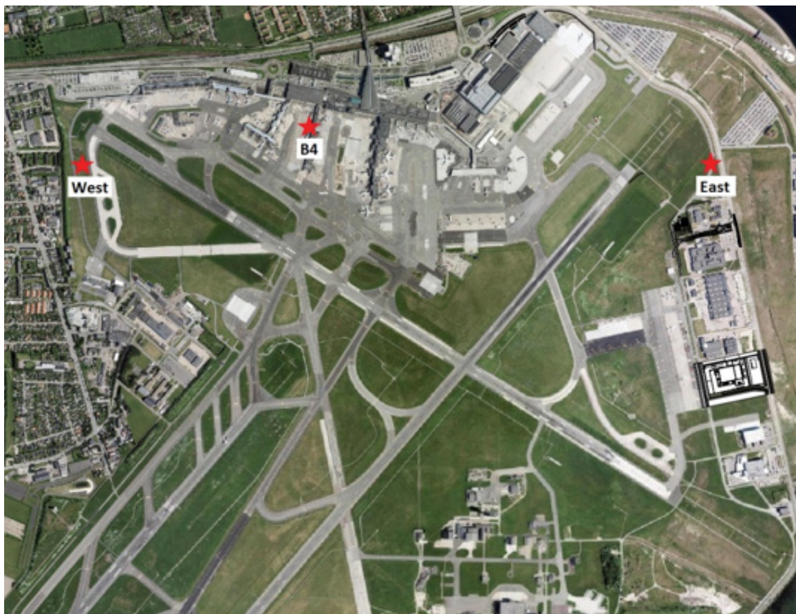
FIGURE 26: COPENHAGEN AIRPORT AND THE LOCATIONS OF THE AIRPORT'S AIR QUALITY MONITORING STATIONS (RED STARS): STATION WEST (NO, NO 2 , PM 2.5 AND UFP), STATION EAST (NO, NO 2 , PM 2.5 ) AND THE APRON STATION, STATION B4 (NO, NO 2 AND UFP).
